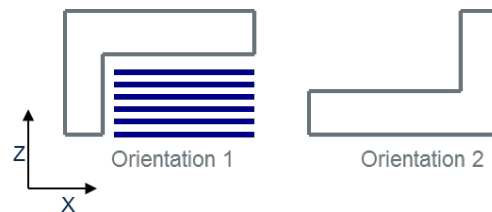
Figure 2: Though identical in Z height, Orientation 2 will minimize build time, reducing support material usage. Also consider, due to the support material interface, the impact on the part's bottom face surface finish.
