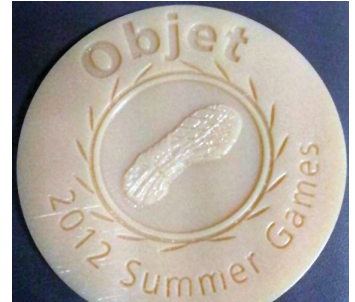
Figure 4: 3D printed model resulting from an STL file made using a BMP image.
